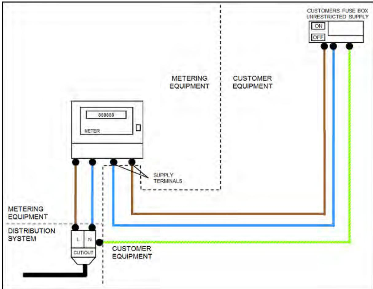
Figure 1 - Typical domestic electrical service position layout<sup>5</sup>
